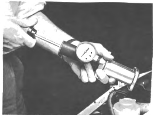
Fig. B:8 Testing the pressure cap
