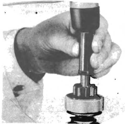
Fig. K:20 Tapping down the circlip retaining ring
