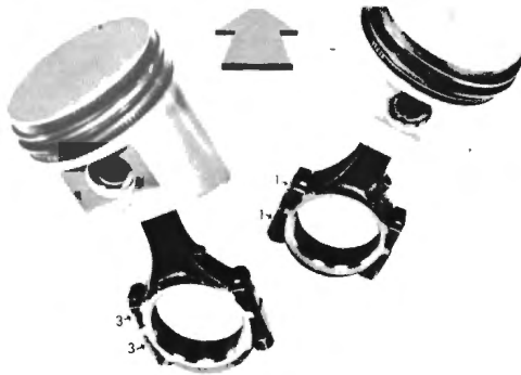
Fig. A:37 Connecting rod and cap numbering
