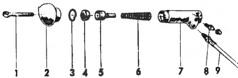
Fig. E:14 Exploded view of the slave cylinder
