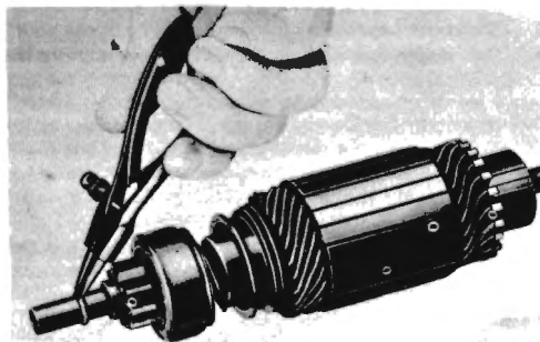
Fig. K:21 Removing the drive pinion circlip
