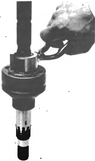
Fig.F:25 Installing the connecting drive shaft in the outer universal joint.
